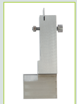
Single shear bearing strength test – procedure C
