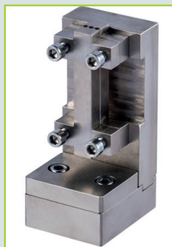
Compression anti-buckling fixture
