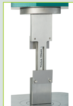
Single shear open hole bearing test fixture – procedure B
