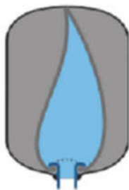
Figure 3.63 Expansion tank with a bladder. Courtesy of TA Hydronics
