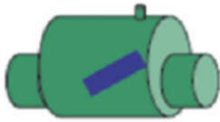
Figure 3.69 Baffle separator. Courtesy of TA Hydronics
