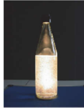
Figure 3.74 Microbubble separation by pressure reduction. Courtesy of TA Hydronics
