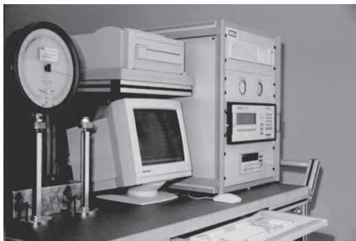
Figure 3.20 Automatic calibration work bench for pressure sensors
