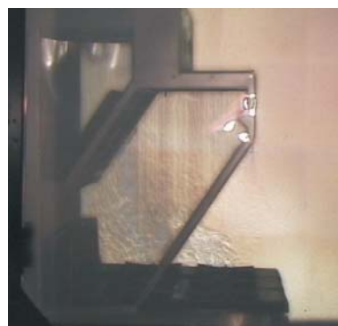
Picture 21. Schlieren Image of KVL Hood. Capture Jet™ On
