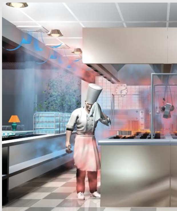
Picture 4. High velocity or mixing ventilation
