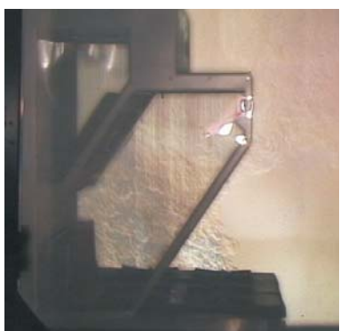
Picture 20. Schlieren Image of KVL hood. Capture Jet™ Off
