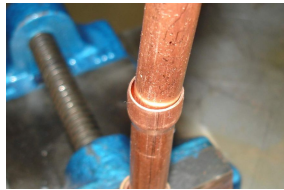
Large clearance results insufficient filling .
