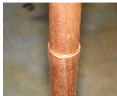
Optimal joint clearance.
