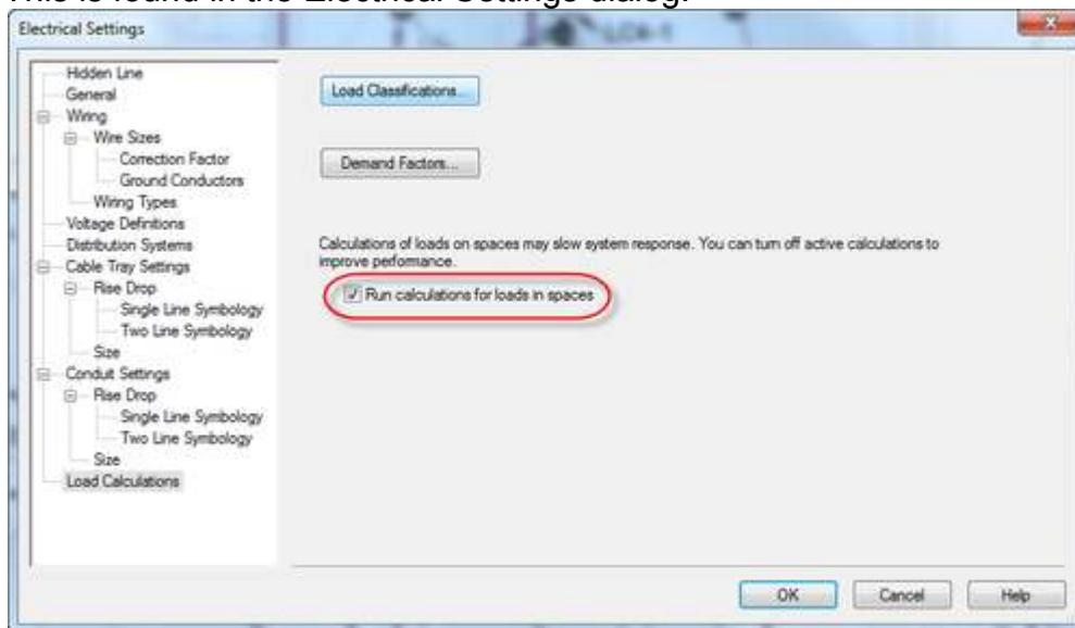
Included in the new Load Calculations panel of the dialog is a control that allows you to turn off load calculations for spaces. Unchecking the "Run calculations for loads in spaces" checkbox will keep Revit from constantly updating these calculations and show the loads as "Not Computed" in the Properties dialog. As soon as the box is rechecked, the values will be calculated again.
