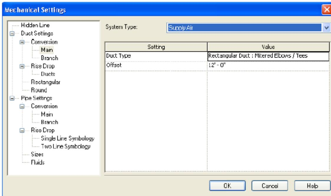
Each system can have its own offset elevation set (which is the relative elevation to the level an item is placed on), so it's a good idea to work out where these areas and elevations will be prior to actually placing any duct or pipe.
