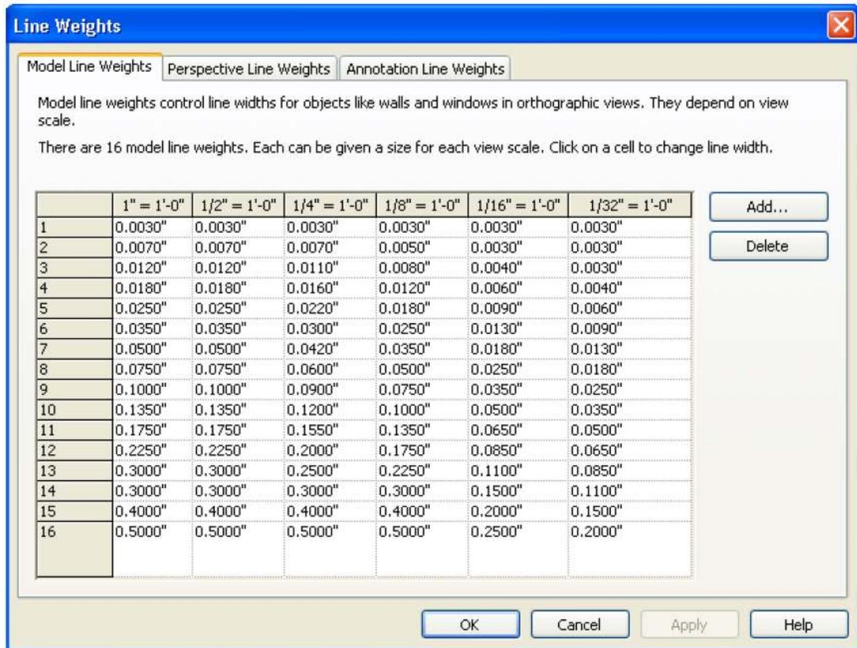
Note how the out of the box settings are defined for model elements – the heavier the weight, the wider the variation between weights in a view, based on scale. The list also leans more towards heavier pen widths, so you can change whole rows at
